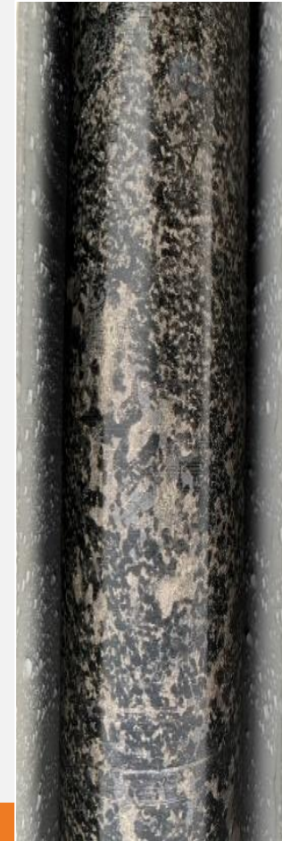
Shallow base metal rich core specimens (G1, G2 and G4 zones)
