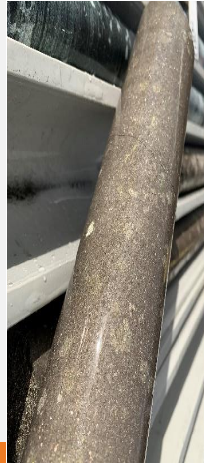
Shallow base metal rich core specimens (G1, G2 and G4 zones)
