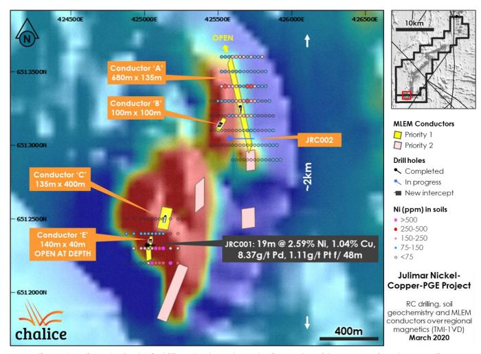
Figure 1. Julimar Project RC drilling, EM targets and soil geochemistry over regional magnetics.
