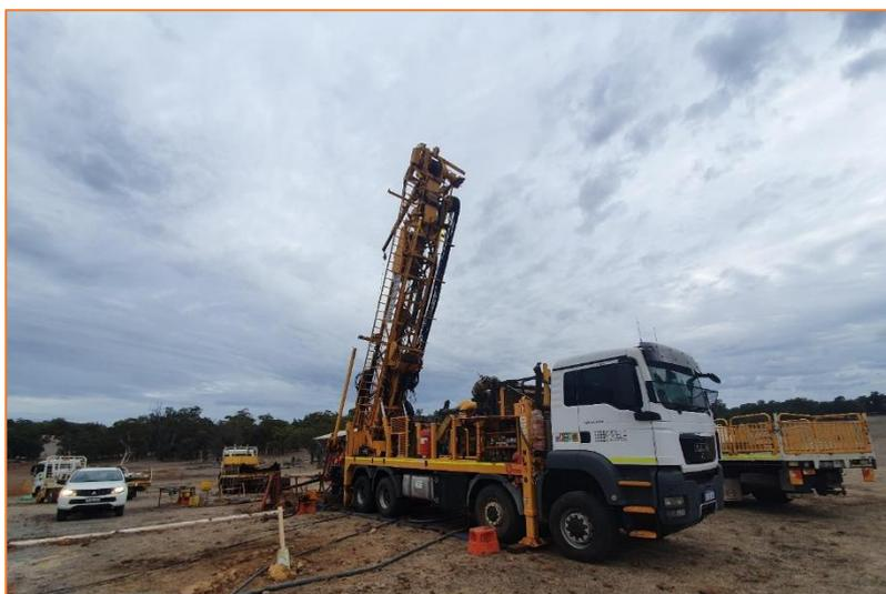
Figure 4. Chalice diamond drilling activity in progress at the Julimar Project
