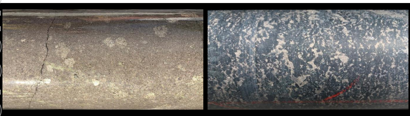
Figure 1. Typical sulphide mineralisation intersected in JD002: hypogene massive sulphides comprising pyrrhotite-pentlandite-chalcocopyrite at ~49.5m downhole (left) and matrix/net textured pyrrhotite-pentlandite-chalcocopyrite at ~90.5m downhole (right). Core photos of entire zone provided in Appendix 1 .
